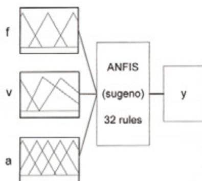
Fig. 2. Fuzzy rule architecture of the triangular membership function
