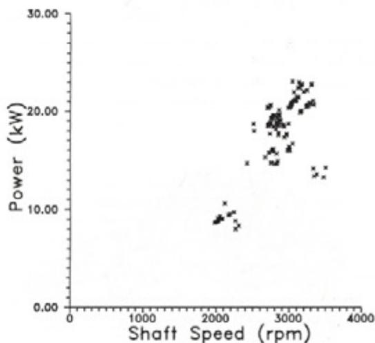
Fig. 8 Expander power output variation with rotational speed
