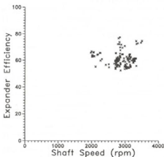
Fig. 9 Expander adiabatic efficiency variation with rotational speed
