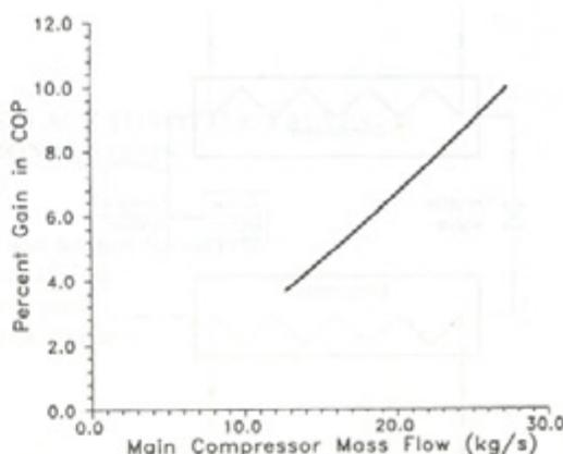
Fig. 3 Gain in COP induced by the expessor
