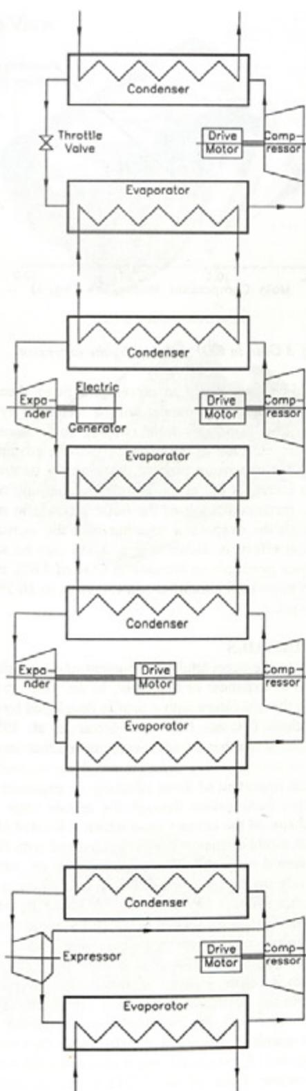
Fig. 1 Chiller unit with two-phase expander as alternative to the throttle valve
