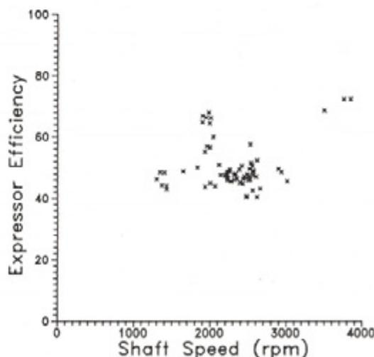
Fig. 11 Expensor adiabatic efficiency variation with rotational speed
