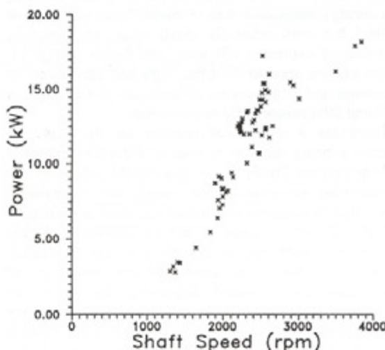
Fig. 10 Expensor power output variation with rotational speed
