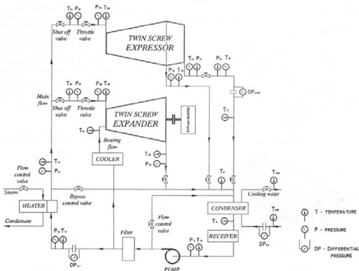
Fig. 7 Expander test rig layout
