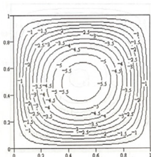
Figure 1; Streamline contours for viscous pseudoplastic fluid for We=0 Ra=10^4 Bi=0
