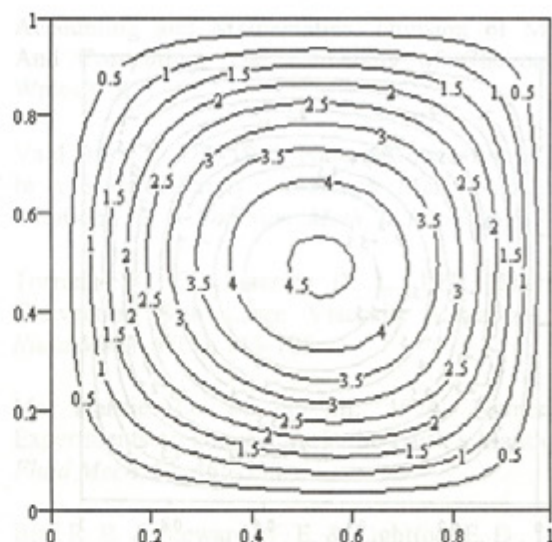
Figure 7; Streamline contours for CEF pseudoplastic fluid for We=0.001 Ra=10^4, Bi=10
