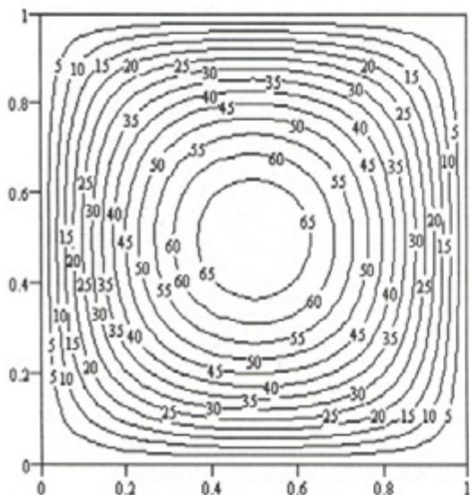
Figure 21; Streamline contours for CEF pseudoplastic fluid for We=0.001 Ra=10^6 , Bi=0
