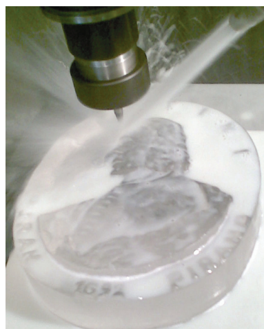
Fig. 18. Physical model manufactured by machining
