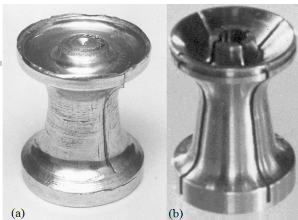
Fig. 1. Axisymmetric part with end thickenings; a) before, and b) after machining
