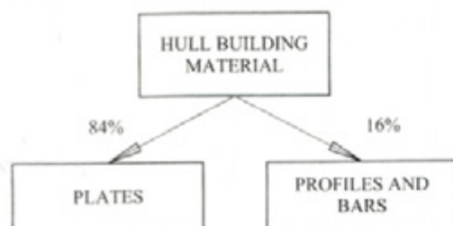
Fig. 3. Mass percentages of plates, profiles and bars in total quantity of material
