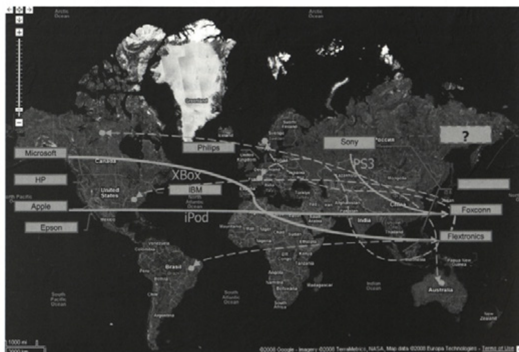
Fig. 8. Design anywhere-build anywhere in consumer electronics: consumers purchase and pay to OEM's (HP, IBM, SONY, etc.), who forward (solid lines) an order-to-build to manufacturers (Flextronics, Foxconn, etc), who ship to customers worldwide (dashed lines). Headquarter locations may change in the near term future; however, the DA-BA principle is not expected to disappear soon.
