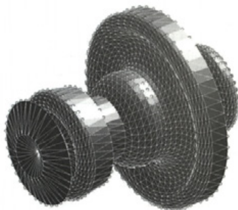
Fig. 1. CAD model example composed from STL triangles
