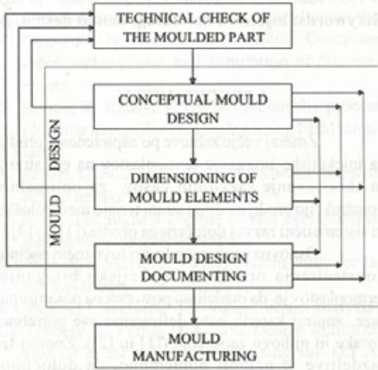
Fig. 1. A shortened diagram of methodical mould design ([1] and [7])
