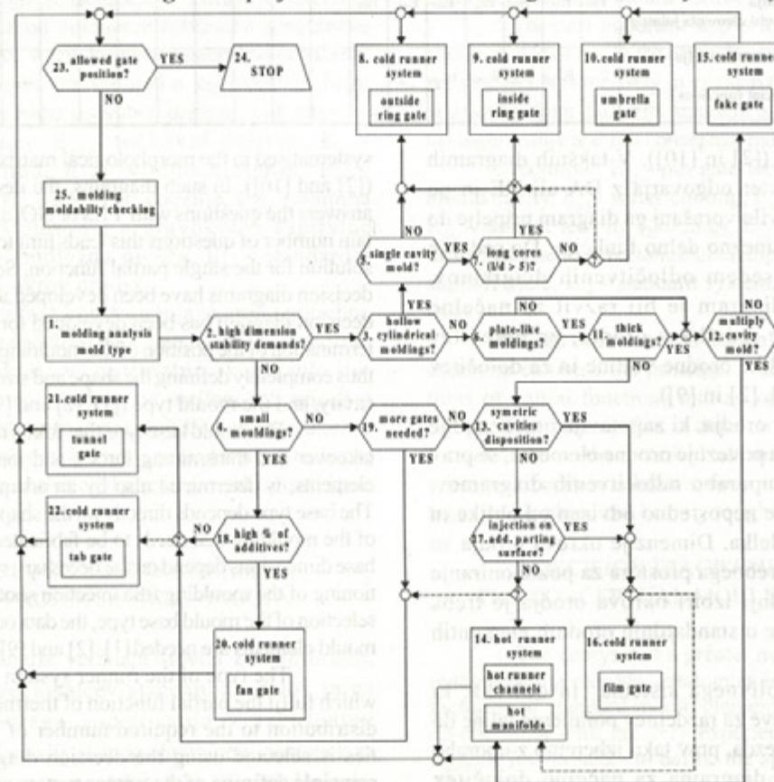
Fig. 3. Decision diagram for conceptual determination of mould runner system and the gate [11]
