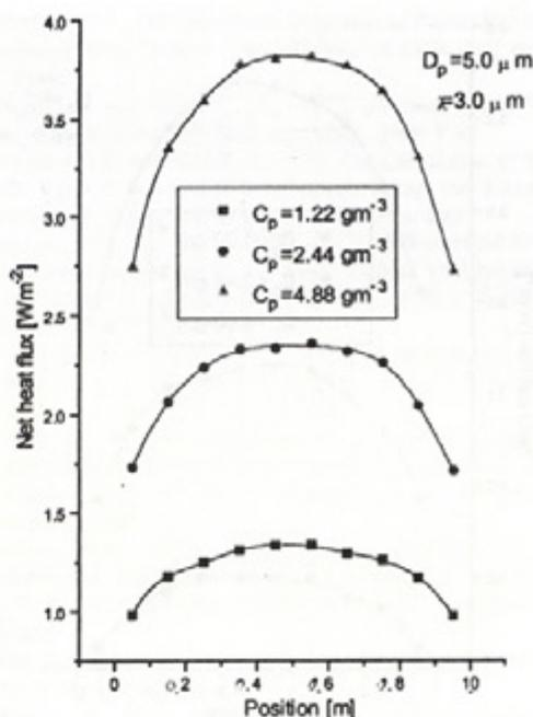
Figure 5. Net heat flux for various particles mass concentrations at wavelength 3.0  $\mu\text{m}$ .
