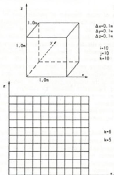
Figure 1. Enclosure geometry and its zoning
