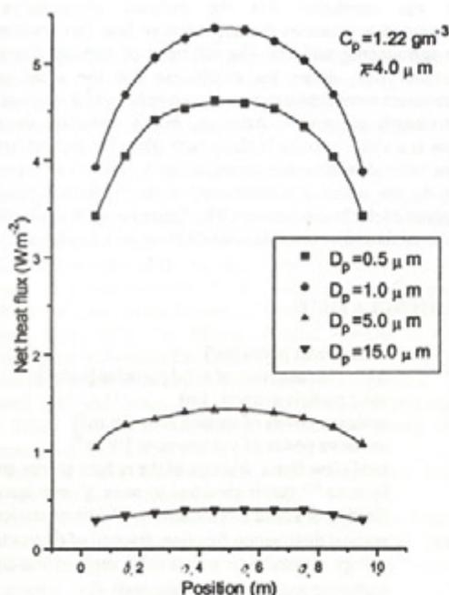
Figure 3. Net heat flux for various particles sizes at wavelength 4.0  $\mu\text{m}$ .
