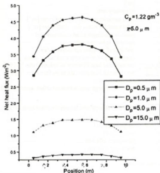
Figure 4. Net heat flux for various particles sizes at wavelength 5.0  $\mu\text{m}$ .
