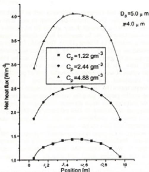
Figure 6. Net heat flux for various particles mass concentrations at wavelength 4.0  $\mu\text{m}$ .
