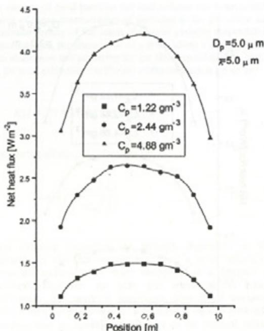
Figure 7. Net heat flux for various particles mass concentrations at wavelength  $5.0 \mu\text{m}$ .
