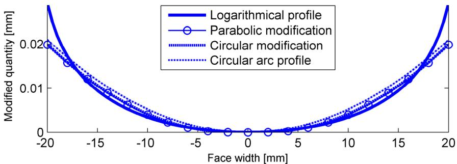
Fig. 3. Optimised lead profiles
